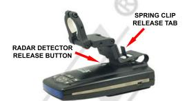
2 - Push the RD release button when installing and removing the RD onto the spring clip. Slide the clip into the RD as far as possible until you hear it lock into position. Remove the RD a few times so you can observe how the spring clip functions. When used properly, the spring clip avoids putting excessive pressure on the mirror stem when installing and removing the RD.
