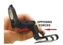
1 - Install your radar detector (RD) onto the mount before installing it on the rear view mirror. To release tension from the spring clip, simply squeeze the release tab and the back side of the mount together. This will lower the bottom portion of the spring clip allowing you to slide the RD on and off the mount.
