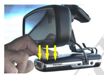
9 - To access the buttons of the RD you will need to gently push downward on the front of the RD with one finger and push the desired button with another finger. Then allow the RD to return to it's original position by gently letting it spring upward. When accessing the buttons, be sure to push the RD downward just enough for your finger to fit between the RD and mirror. Do not push down more than what is needed.
