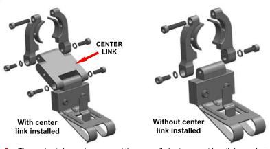
5 - The center-link may be removed if an overall shorter mount length is needed, depending on your rear view miror and desired position for the radar detector.
